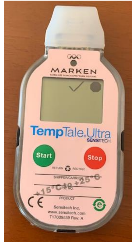
TT4 stopped, no alarm.
